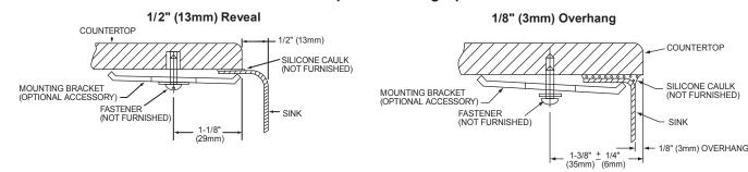
NOTE: THIS UNDERMOUNT SINK IS DESIGNED TO MOUNT TO SOLID SURFACE (NON-LAMINATE) COUNTERTOP ONLY.
